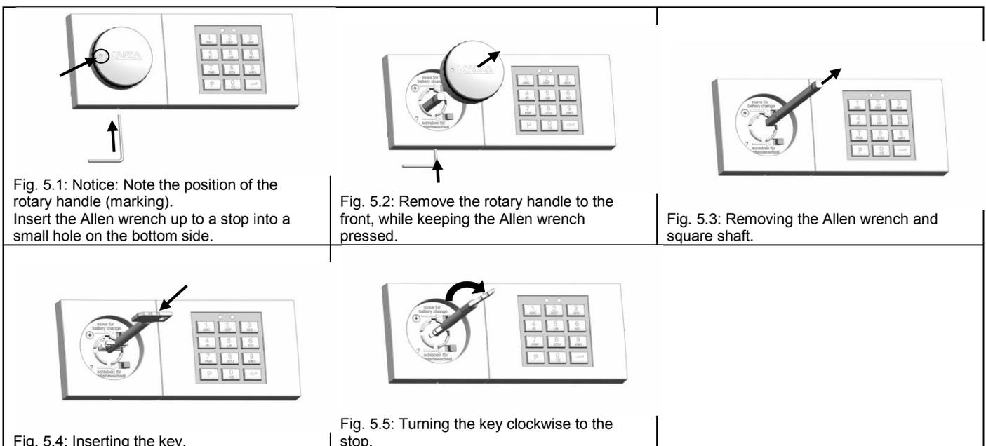
Figure 13: Opening with the key
