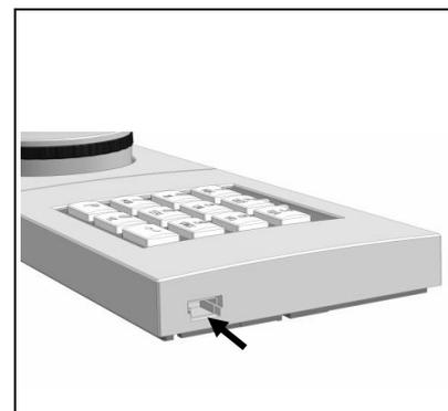
**Figure 10: Mini-USB socket**
