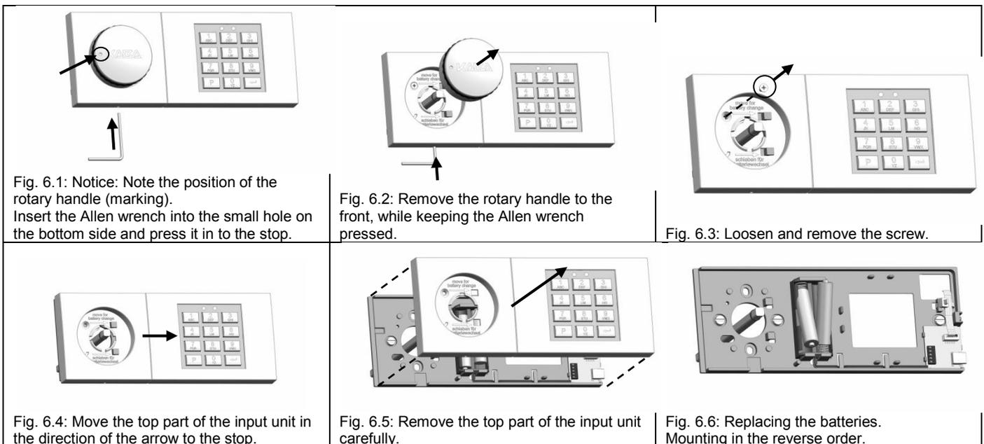
**Figure 14: Battery replacement**
