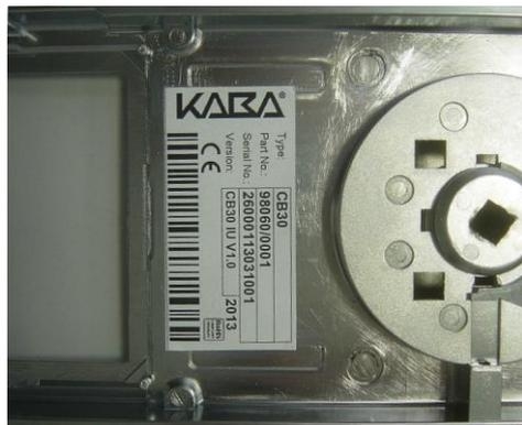
Figure 15: Label with the production data in the input unit
